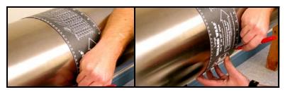
Figure 3-5: Measuring and Marking Circumference Lines
